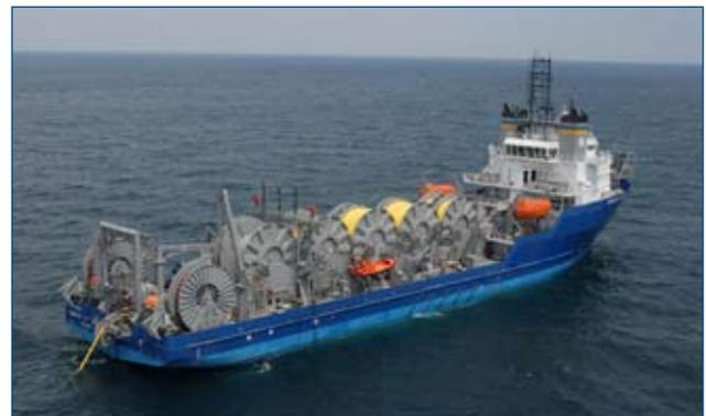
*Military Sealift Command ship named VADM K.R. Wheeler after the 31st Chief of Supply Corps is an offshore petroleum distribution system that pumps fuel ashore from up to eight miles at sea.*
